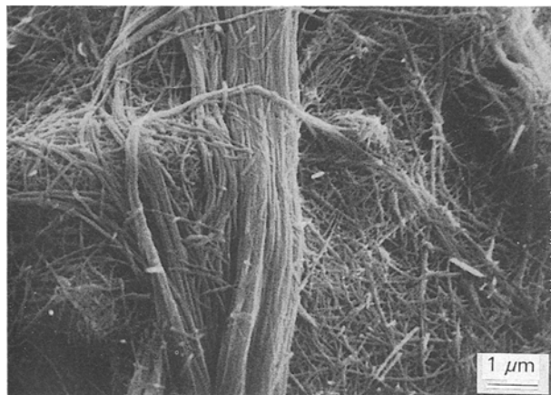
Figure 6 Calcium germanate hydrate formed at 5°C is typified by tightly matted fibres.
